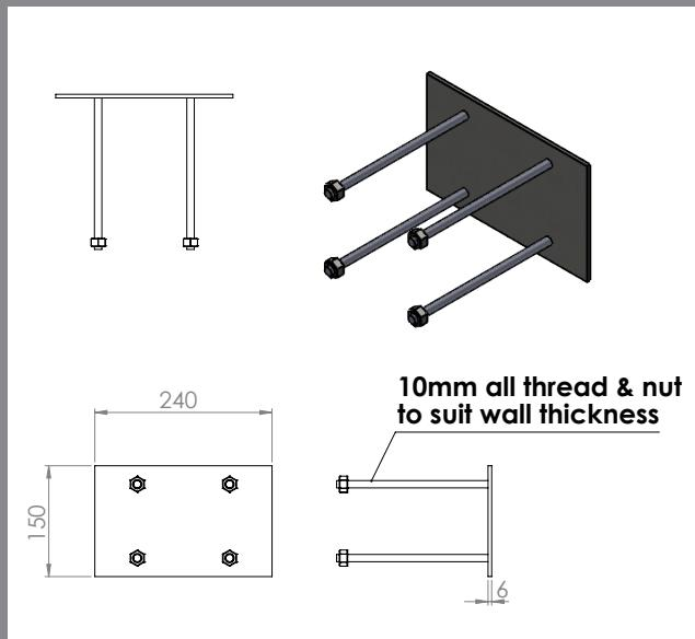
Accessory to be used with the SCEC-approved G-KC1 Safe. Installation of the G-KC1 is in accordance with working note 1-84.
