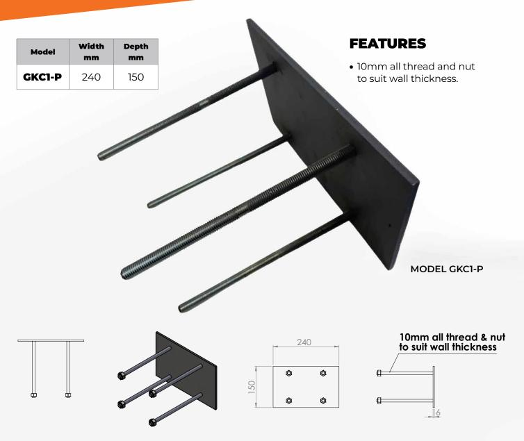
Accessory to be used with the SCEC-approved GKC-1 Safe. Installation of the GKC-1 is in accordance with working note 1-84.
